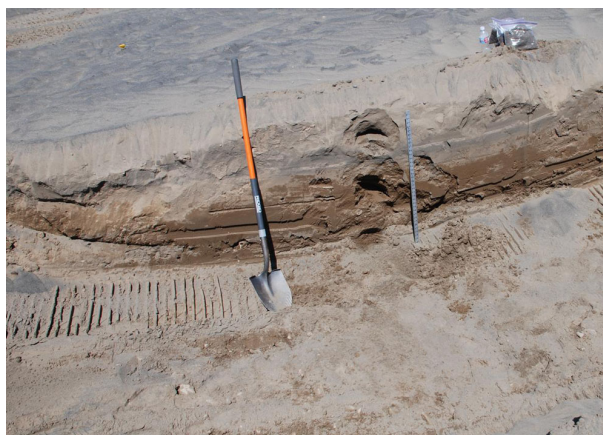
Figure 9. Excavated trench reveals layers of wet clays and alluvium beneath Moses Lake Sand Dunes
