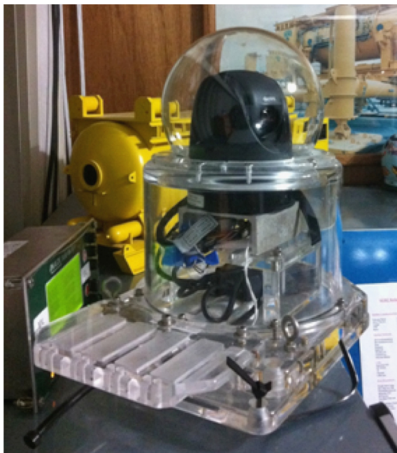
Fig. 28. Underwater Gigapan Voyage unit for NEEMO 15.
