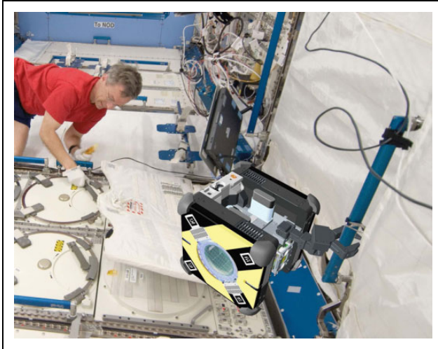
Figure 3. Artist's concept of the Astrobee robot taking video of an astronaut activity while perching.
