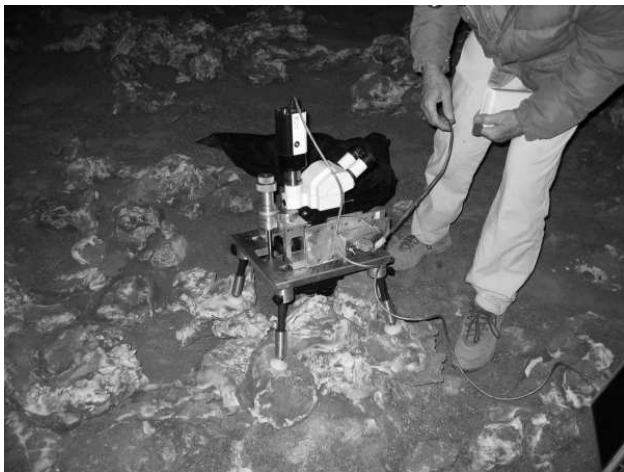
Figure 2. (above) colored LEDs provide illumination for a nighttime fluorescence imager test; (below) a backpackable fluorescence microscope was used for ground truth
