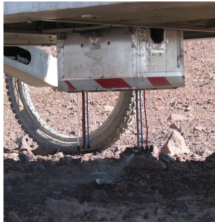
Figure 8.4: The microscopic fluorescence imager deployed and spraying underneath the robot.
