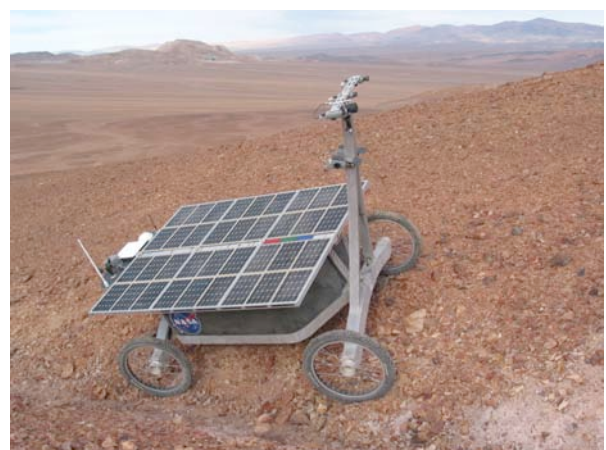
Fig. 4. Zoë climbing a cross slope in the Atacama Desert. Maximum slope climbing capability reaches the angle of repose of unconsolidated sand, about 30°.
