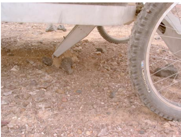
Fig. 5. Plow prototype deployed under the rover overturns the top 2 cm of material as Zoë moves backwards (toward right) to image exposed subsoil that it imaged undisturbed while moving forward.
