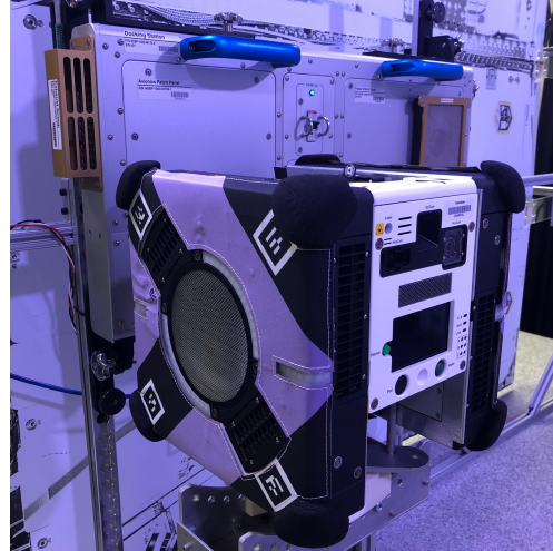
Fig. 1. Astrobeer docking on the station on the top of micro-gravity simulating surface.
