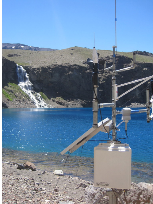
Figure 3: Backup meteorology station on the shore near the LakeLander. This station includes additional sensors for measuring precipitation, solar insolation, soil temperature and lake level.
