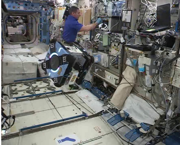
Figure 2 Bumble moves into position for its targeted inspection during the fault management scenario. Astronaut Mike Hopkins is seen working in the background.
