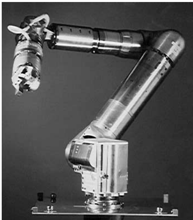
Photograph of SPIDER, the teleoperated robotic arm designed by the Agenzia Spaziale Italiana (ASI).
