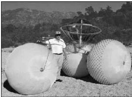
One model of an inflatable rover, JPL's design for traversing rugged terrain.
