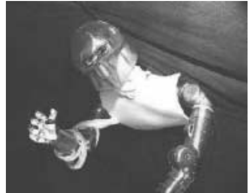
Photograph of Robonaut, with dexterous arms and hands to assist astronauts.
