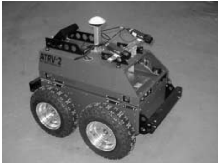
The Bullwinkle rover, used as a test platform for the Mars Autonomy project path planner.
