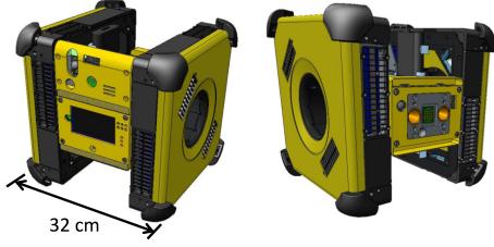
Fig. 1: Picture of Astrobee: A free flying robotic platform being designed for zero gravity flight inside of the International Space Station
