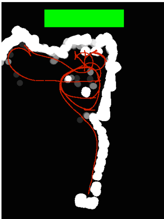
Figure 4. Navigation map from an traverse on a promontory (in Pittsburgh). The goal is the rectangular region at top. Round dots in varying size and shades of grey indicate obstacles. Zoë circles around as it seeks a path down off the promontory to the goal. Note several points where the rover backed up. This pathological case ended when Zoë ran out of time to reach its goal.
